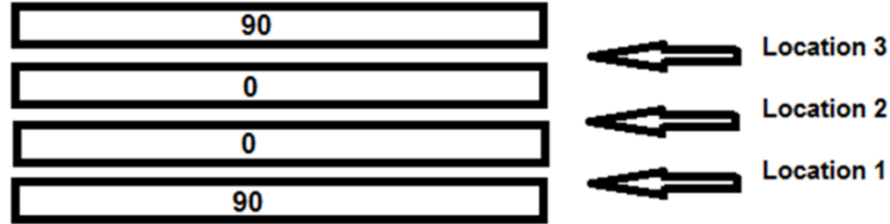
Figure 4.2. Specimen layup and planned delamination locations.
