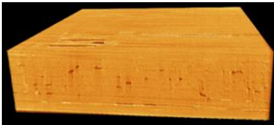
Figure 4.11. 4X 3D X-ray image of cross-ply specimen subject to 12000N tensile force (Matrix Damage present)
