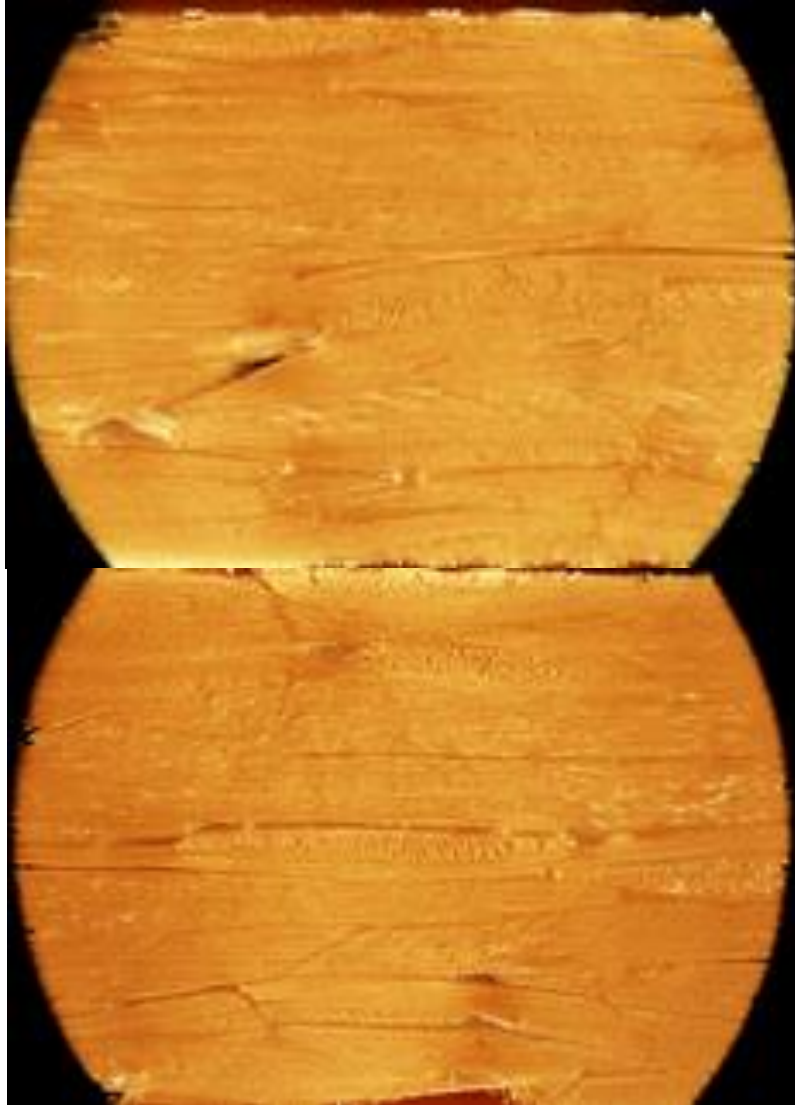
Figure 3.7. 3D X-ray images (4X magnification) of quasi-isotropic carbon fiber specimens impacted at 16J (above) and 18J (below)
