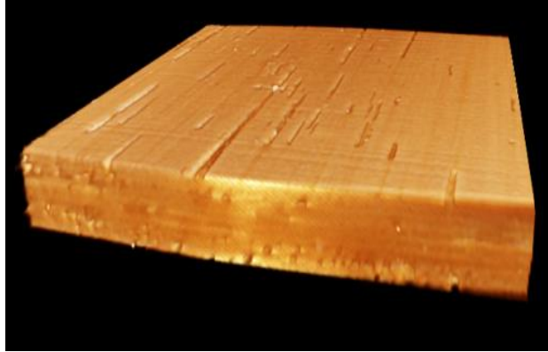
Figure 4.10 1X 3D-Xray Image of cross-ply specimen subject to 12000N tensile force
